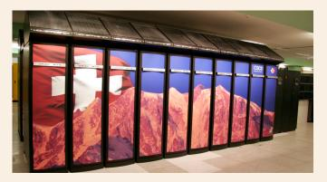
Monte Rosa is the largest production system at CSCS and will be upgraded in October 2011 to AMD Interlagos 2 x 16-core 64-bit CPUs, 32 GB per compute node, and high performance networking with Gemini 3D torus interconnect. It features a total of 1'496 nodes, that is 47'872 cores.
