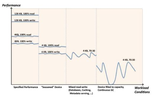
Figure 2: Performance variations in current generation of NAND Flash---based SSDs [taken from 1]
