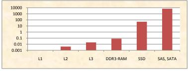
Figure 1: Typical latency in µs for several storage devices
